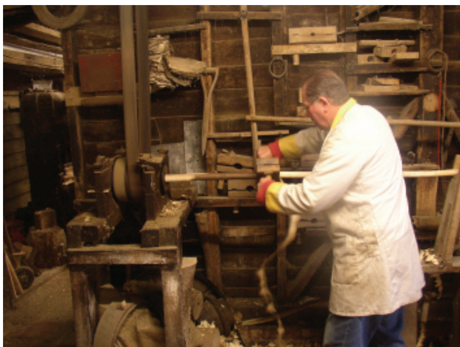
Smoothing the rake handle using a semi-automated device in the old workshop at Smeeth
