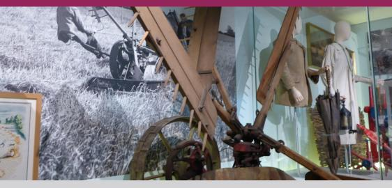
**Key information** This machine used to cut crops in the field using the rotating arms. People would follow this machine gathering, binding and threshing the crops.
