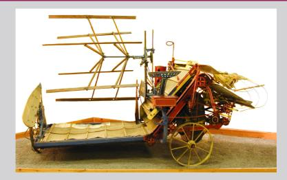
**Key information** This harvesting machine used to cut crops and bind them into bunches as it travelled across a field.
