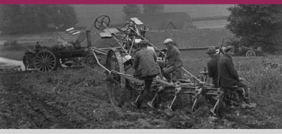
**Key information** John Fowler invented the steam plough. He set up a steam engine at each end of a field. These would then draw a plough across the field by a cable. Usually this was operated by a team who lived and travelled together in a van containing all the equipment.
