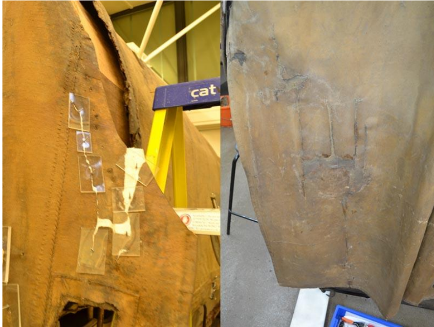
Left: repairs to tears in the canvas tilt underway, using calico and a Perspex clamping system. Right: canvas tilt repairs completed and colour-matched ready for redisplay (MERL 51/1295).
