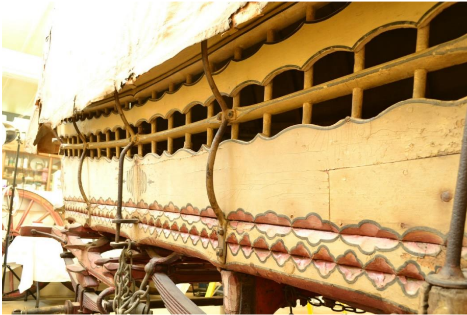
Detailed image taken during conservation showing the side panels and iron straps, and the relatively light construction of the vehicle (MERL 51/1295).
