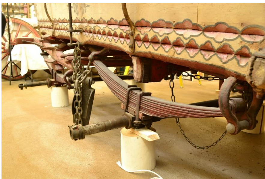
Detailed conservation image showing decorated side panel, springs, and rear axle. Note the strap on timber above the spring; this acts as a stop to limit travel and thus prevent breakage of springs (MERL 51/1295).
